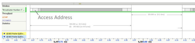
Figure 10 Broadcast Packet with Access Address Field Highlighted.
